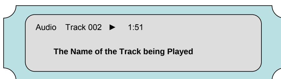
Figure 2-34 – Application Example of Track/Chapter Name Display on constrained device
